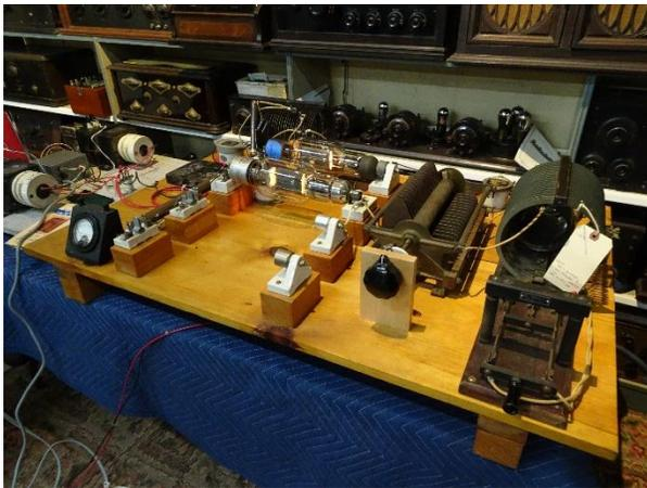
The plan was for the replica transmitter to be operated during the evening as W2AN/1BCG on 1.821 MHz, plus or minus, using CW. Members of the RSGB in Ardrossan were listening for those signals with the goal of replicating the 1921 successful transatlantic reception using a 1921 designed transmitter.
